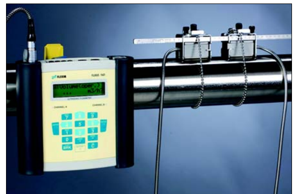
Measurement with transducers mounted by fastening shoes and flow transmitter fixed to the pipe by the QuickFix pipe mounting fixture
